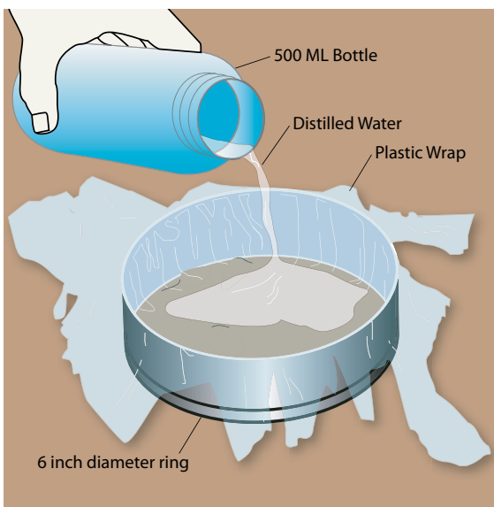
Figure 2 Pour the 444 mL of water (1 inch of water) into the ring lined with plastic wrap.
